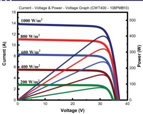
The specifications are obtained under the standard test conditions: 1000W/m2 solar irradiance, 1.5 Air Mass and cell temperature of 25°C. Measurement uncertainty for all panels is 3%. The actual transactions will be subject to the contracts. These parameters are for reference only and it is not a part of the contracts. The technical specifications in this document may vary. For more information, refer to the "Installation Manual".
